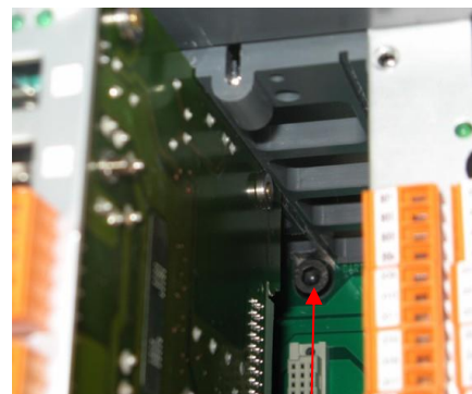
Mounting screw 4 Below module slot 1xx (the power supply unit must be removed to release it).
