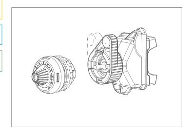
Mounting the potentiometer for railmounted:
