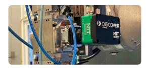
DISCOVER IR SUITE provides, in-process, quality assessment (Ok, NOk)\*\* of a brake disc coating process.
