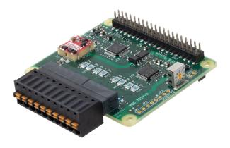
This product is an expansion card that adds a thermocouple interface to the Raspberry Pi.
